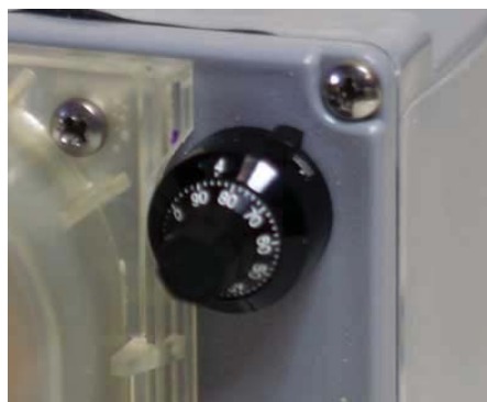
Optional 10-turn potentiometer for finer flow control.
