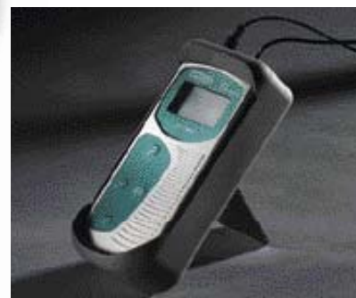
Left: pH 6 portable meter shown with pH electrode 35801-00 and temperature probe 35613-05.
